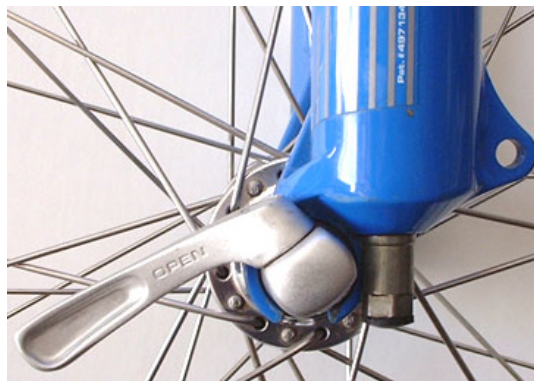
Read the lever to tell if it's safe. If it reads "open," the wheel can come off!!
